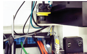
Vision system ( above ) triggers job change and maintains registration. Roll feed ( right ) helps optimize digital converting investment.
